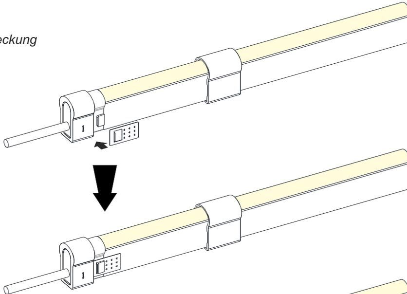
Push Pc cover over anti-skidding clip onto the assembly end of the light. /
