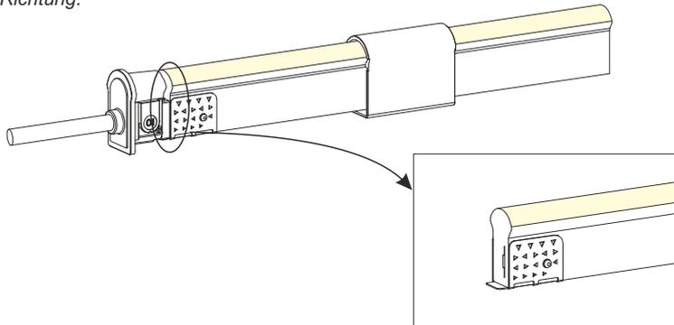
Fit the anti-skidding clip to the end of the light so that it wraps tightly and
