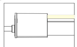
Slide back the PC cover till it snaps in the feed connector. /
