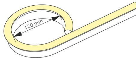
Do not bend smaller than allowed minimum bend diameter 120mm.
