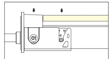
Press the feed connector and tube downwards at the same time till bottom. /
