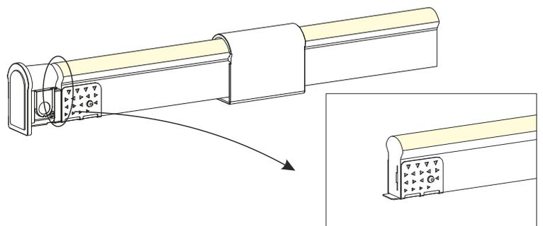
Fit the anti-skidding clip to the end of the tube so that it wraps tightly and its brim is
