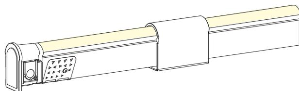
Place the anti-skidding clip onto the assembly end of the tube. Pay attention to its direction. /
