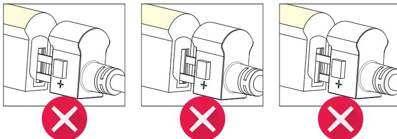
Insert into the front side of the PCB /
