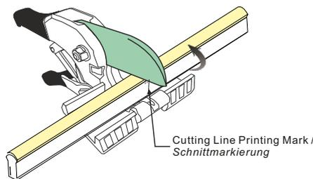
Printing mark should be faced upwards. /
