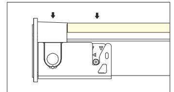
Press the tail plug and tube downwards at the same time till bottom. /
