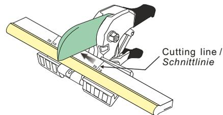
Cutting can only be made at the printed cutting line. /
