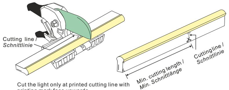
Cut the light only at printed cutting line with printing mark face upwards.
