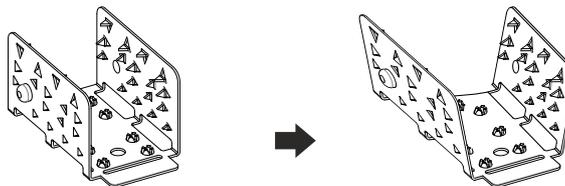
Unfold the anti-skidding clip about 20 degrees
