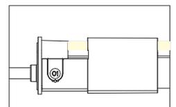
Please energize the tube to check its functionality and do waterproof reliability testing after connector assembly.
