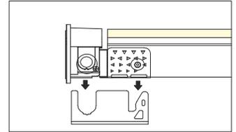
Align the tail plug and anti-skidding clip with the U steel plate. /
