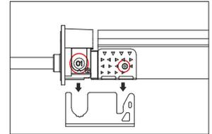
Align the feed connector and anti-skidding clip with the U steel plate. /
